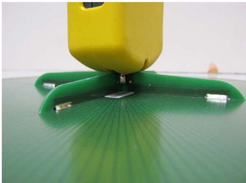
The "official" TCO guideline can be found under [www.TCODevelopment.com](http://www.TCODevelopment.com). The measurement should be performed with a **grounded** instrument at a distance of 30 cm towards the item to be evaluated.
