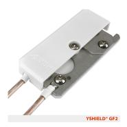
Medium-sized surface/flash mounting housing 40x80 mm, for the installation directly on shielding products or for clamping the grounding straps. With a clamping point for grounding straps preferably for small surfaces with shielding paint, shielding mesh, shielding plaster, reinforcement fabric. Usage on the interior as well as the exterior (additional seal necessary). One piece is needed per surface. Flush mounted with a height of 11 mm is thinner than a drywall construction board.
